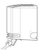
**4** Press and hold the **Ϡ** button for about 5 seconds to close the air deflector.
