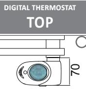
The general footprint has to be calculated considering the thermostat height
