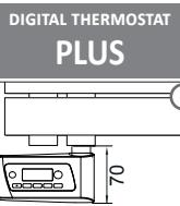
The general footprint has to be calculated considering the thermostat height
